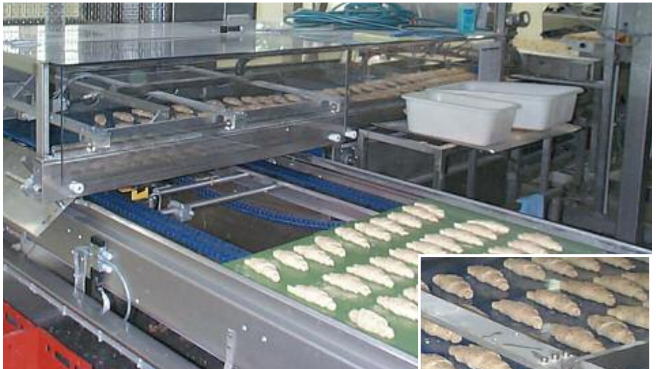
This application from the food industry transfers breads and pastries from one conveyor to the next. Lubrication is totally prohibited due to food contact. Another reason for using the DryLin® R linear plain bearings is the resistance to corrosive cleaning agents. Additional benefits include the reduced design space required by the iglide® J bearings and the excellent corrosion resistance.
