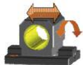
The self-aligning DryLin® R bearings of the 06 LL design series can compensate parallelism errors up to ± .12" (3mm).
