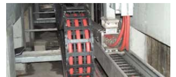
Floating towing arm, to counter misalignment
