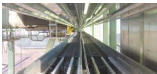
Extension link support for E-ChainSystem® with several extension links
