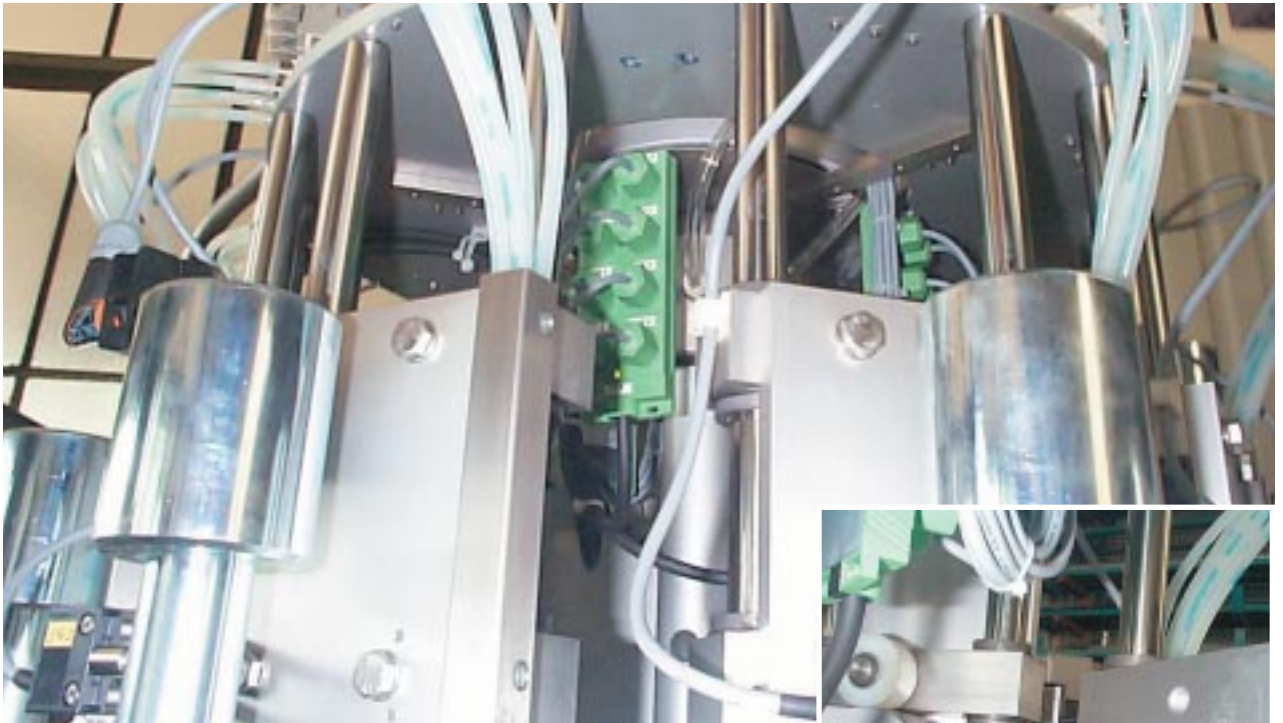
This application, a rotary transfer machine, seals champagne bottles with corks, aluminum caps and wire braid. The fact that the DryLin® guide systems are lubricant free is important in the food sector, additional benefits include resistance to chemicals and cleaning.
