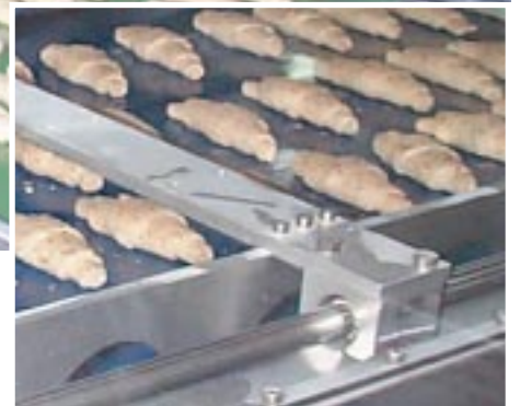
This application from the food industry transfers breads and pastries from one conveyor to the next. Lubrication is totally prohibited due to food contact. Another reason for using the DryLin® R linear plain bearings is the resistance to corrosive cleaning agents. Additional benefits include the reduced design space required by the iglide® J bearings and the excellent corrosion resistance.
