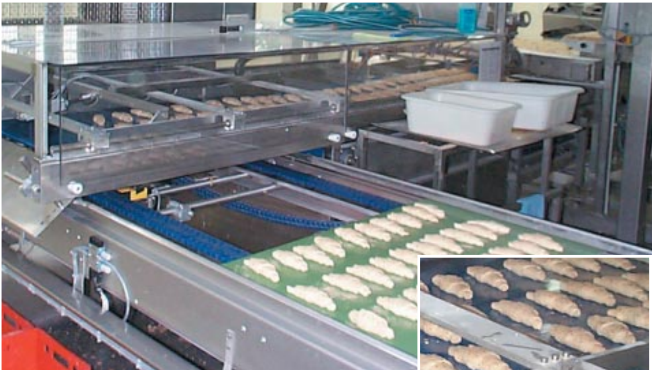
This application from the food industry transfers breads and pastries from one conveyor to the next. Lubrication is totally prohibited due to food contact. Another reason for using the DryLin® R linear plain bearings is the resistance to corrosive cleaning agents. Additional benefits include the reduced design space required by the iglide® J bearings and the excellent corrosion resistance.
