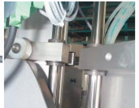
This application, a rotary transfer machine, seals champagne bottles with corks, aluminum caps and wire braid. The fact that the DryLin® guide systems are lubricant free is important in the food sector, additional benefits include resistance to chemicals and cleaning.
