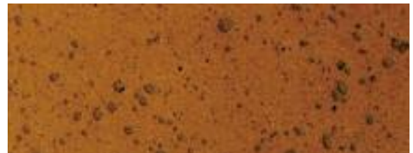
Base plastics without reinforcing materials with solid lubricants, magnified 200 times, dyed.
