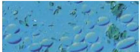
Base plastics with fibers and solid lubricants, magnified 200 times, dyed
