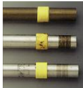
Wear experiments with aluminum shafts
