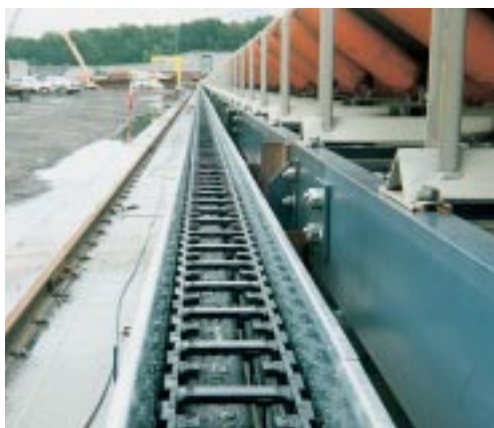
Conveyor belt in quarry. Travel distance of 587 ft (179 m), travel speed 220 ft/min. (67 m/min.) and fill weight 5.38 lbs/ft (8 kg/m)
