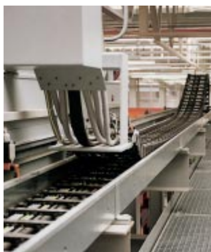
Robotics: quiet running, high acceleration; up to 10,000 cycles per day
