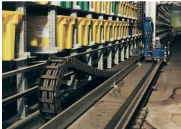
Automated storage/retrieval system with System E2 and Chainflex® cables - travels up to 80 m and speed of 14.8 ft/s (4.5 m/s)
