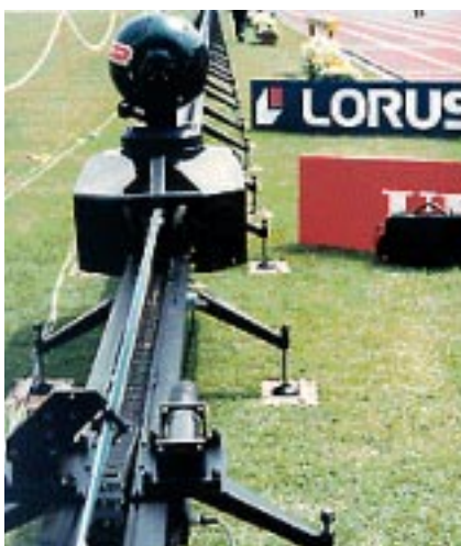
Mobile camera, live images, Olympic Games in Atlanta S = 328 ft (100 m) V = 32.8 ft (10 m/s) in push-pull operation
