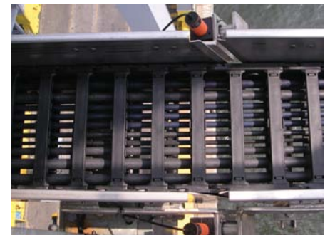
Hinge clutch at the hinge point with a limit switch for connection control.
