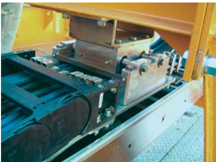
Floating moving arm on "ship-to-shore" crane compensates for lateral mismatch between trolley traveling path, crane traveling path and the pre-harnessed cable carrier systems. Electronic push-pull force control with nominal/actual parameter check and emergency stop function optional.
