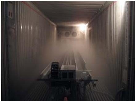
Climate tests for Energy Chains® and Chainflex® cables in temperatures from -40° F up to +390°F
