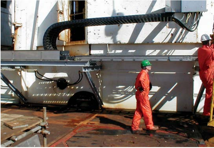
Lightweight and high stability: Short/cross travel application with Series E4/4 guided in a stainless steel guide trough
