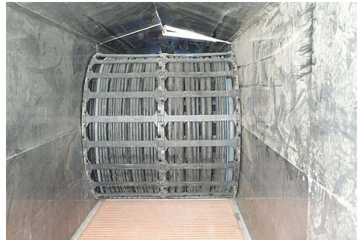
Series 600 with extension link in igus® specially designed guiding channel in the Caspian Sea
