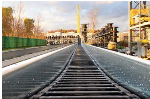
This flagship application, to test long travel applications up to 410 ft and speeds of up to 984 ft/min., has been running for 4 years
