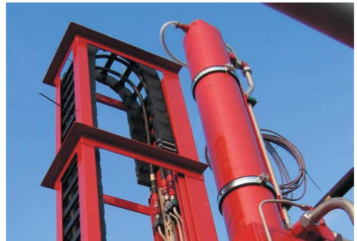
Vertical boom on a riser-handling crane for AKMH (West E Drill)
