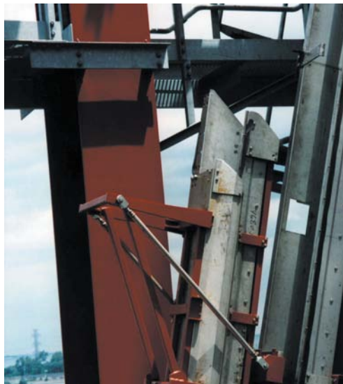
To make sure the boom and the girder sides of the crane are connected without misalignment of the guide trough, igus® developed a special fixing for the swivel point. This means that the carrier can run on top, beside or below the crane girder.
