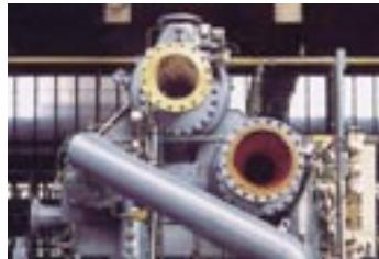
Picture 13.1: Intake control device
