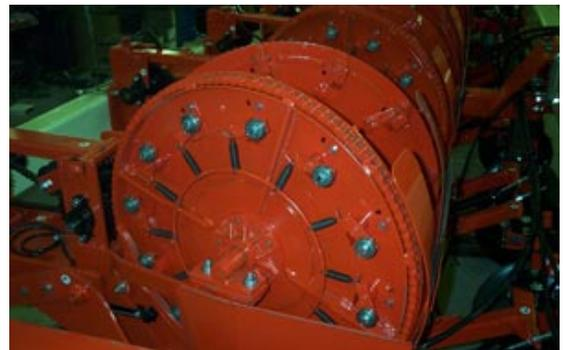
A planter pick arm was encountering several problems due to the oil-impregnated bronze bushings with graphite plugs used. The pick arm rotates through an arc of 15% at a rate of 12-20 cycles per minute. On the West coast, the bronze bearings were experiencing high wear and premature failure due to very abrasive conditions caused by high levels of volcanic ash in the soil. On the East coast, high salt content in the air caused corrosion and seizure.
