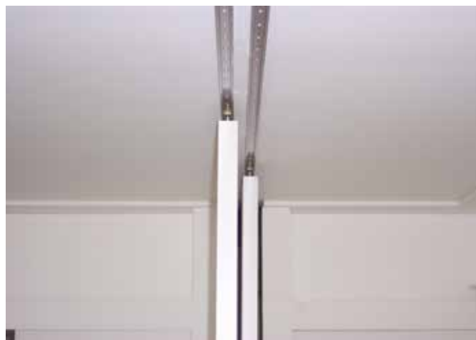
The quiet, self-lubricating, and low-profile design of DryLin® N enabled it to fulfill the safety requirements of this application. Multiple sections of rails are joined to achieve the desired length.
