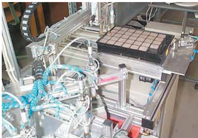
The removal unit is moved along the X-Y axis using space and cost-saving DryLin® N.
