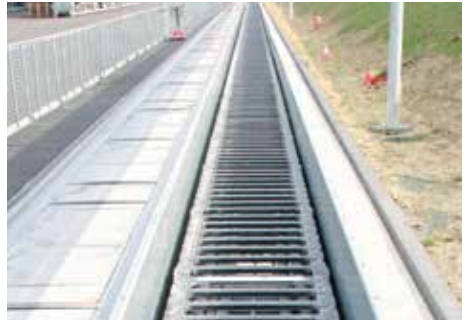
P4-56: igus® outdoor testing - travel length 394 ft.
