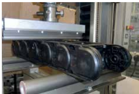
Strength test: calculation of the maximum unsupported length
