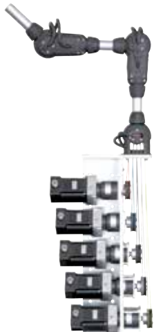
robolink drive unit for a 5 DOF articulated arm
