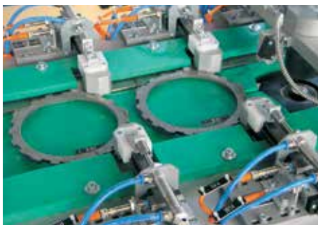
drylin® test station for the eddy-current crack test of components for the automobile industry
