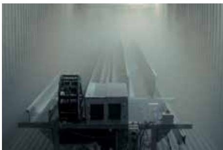
Frost test: Cables and e-chains® at -40°F
