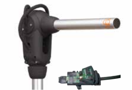
robolink joint – optional with angle sensors
