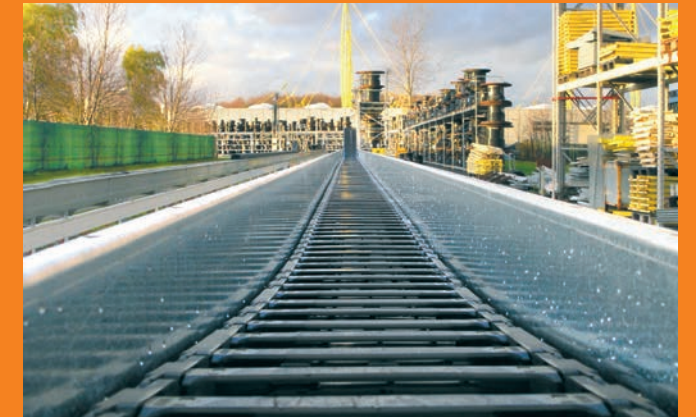
Long travel test facility - 125m travel length, speed 300m/min
