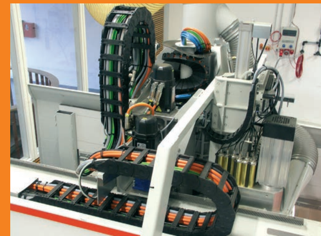
An igus® twisterband guides the energy of the 5-axis cutting head in this wood working machine, safe and cost-effective
