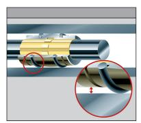
DryLin® R-03 bearings can compensate for parallelism errors using O-rings
