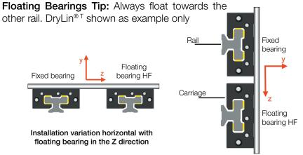
Installation variation lateral with floating bearing in the Z direction
