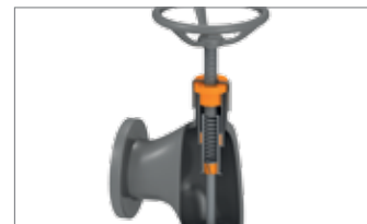
Lead screw nut in block valve
