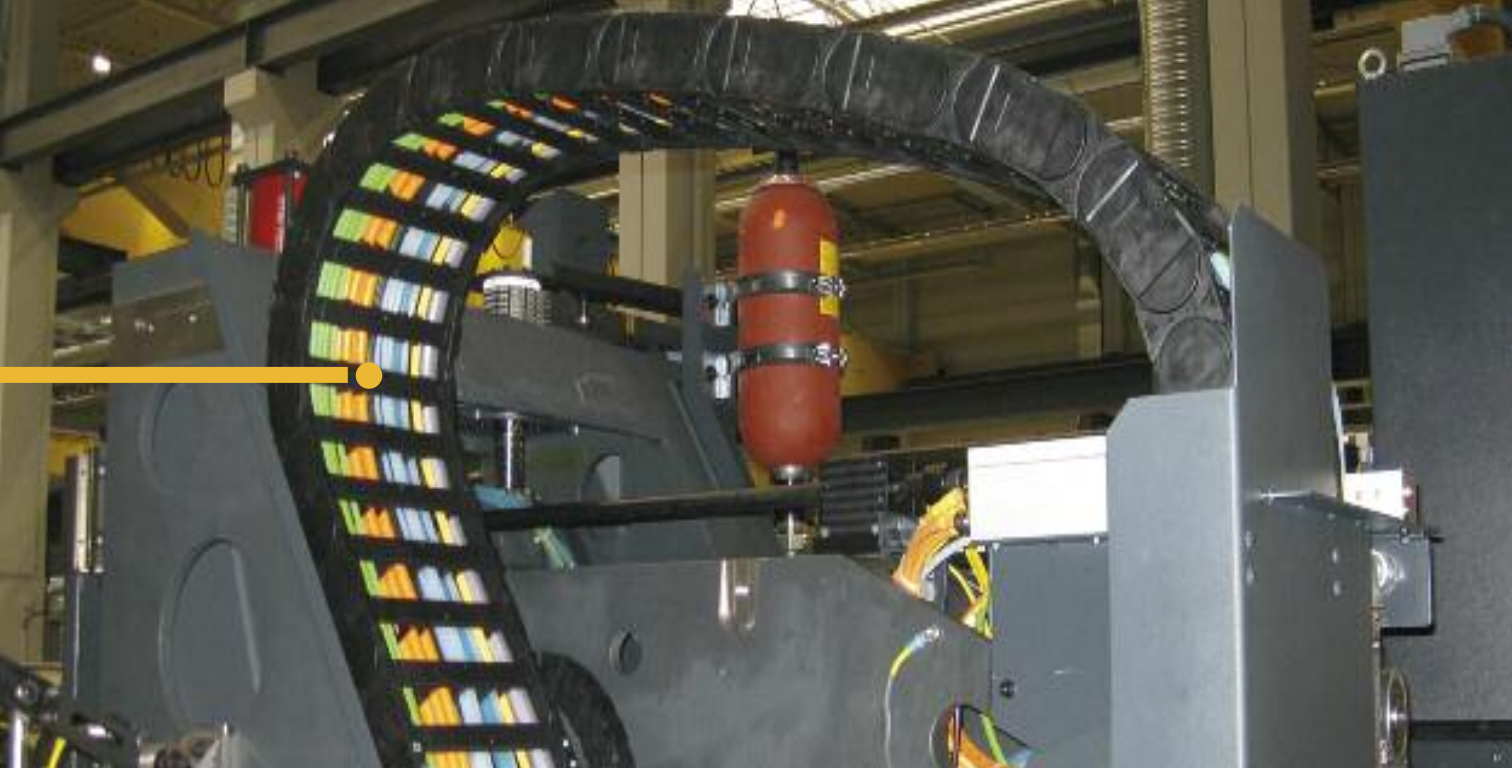
The E4-42 series in a machine tool, completely assembled with igus® Chainflex a cables
